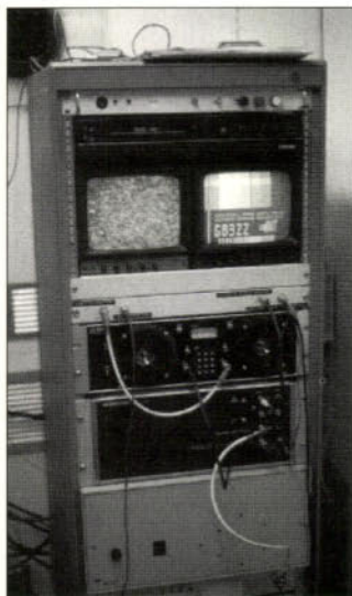
An actual 1.3GHz ATV repeater in service. This very professional-looking hardware is GB3ZZ in Bristol, run by the Severnside ATV Group.
