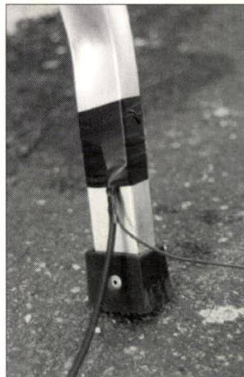
Fig. 6: Connections to the vertical antenna. The wire radial is connected to the outer of the coaxial cable and must be insulated from the antenna.
